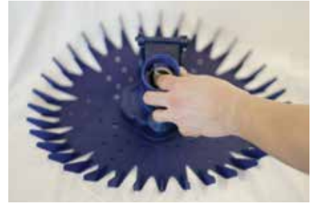
Step 3 Squeeze top edge section of diaphragm together and push down.
