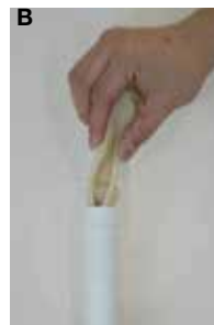
Insert folded top edge of diaphragm into inner extension pipe as in diaphragm B.
