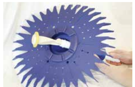
Step 6 Turn cleaner body upside down insert inner tube with diaphragm and pull through cleaner body until the diaphragm pops in and releases from inner extension pipe.
