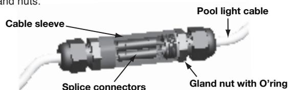
*Note: If the power cable is 6mm diameter use the smaller joiner tube and gland nut assembly.*
