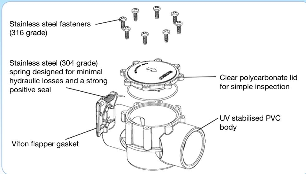
The Flow Check valve's pressure rating of 400 kPa (58 psi) and its 316 stainless steel fasteners make it suitable for domestic and commercial applications.
