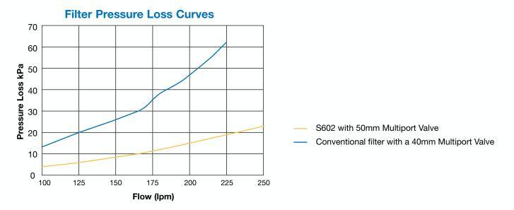
The Micron S602's design combined with its 50mm Multiport valve reduces its pressure loss from 60 kPa (@ 225lpm) down to a very low pressure loss of 20 kPa (@ 225lpm).
